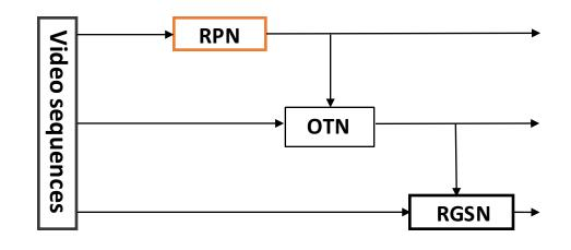
The Region Proposal Network is pre-trained on COCO and provides class-agnostic object candidate boxes. RPN could encode the instance(object) information into framework.
