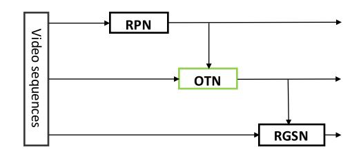
Inspired by MDNet, Object Tracking Network is designed to score the candidate boxes and updated online for adapting to large and fast changes in object appearance.
