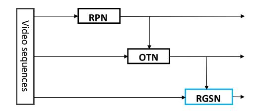
Then, the box with the highest score evaluated by OTN is selected to crop and resize the frame for normalizing the scale variation of objects.
